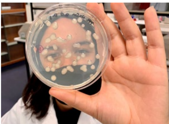
PhD student Crystal Young screening microbial populations for their ability to produce compostable bioplastics
